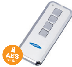
Handsender Mini-Novotron 524 Design 4-Kanal, 433 MHz, KeeLoq-Wechselcode
